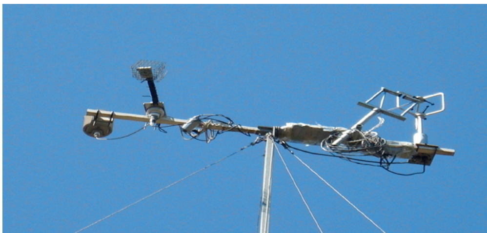
Fig. 2a: The ISAC base : particular of the mast top: from left: thermohygrometer, net radiometer, surface temperature sensor, fast krypton hygrometer, ultrasonic anemometer
