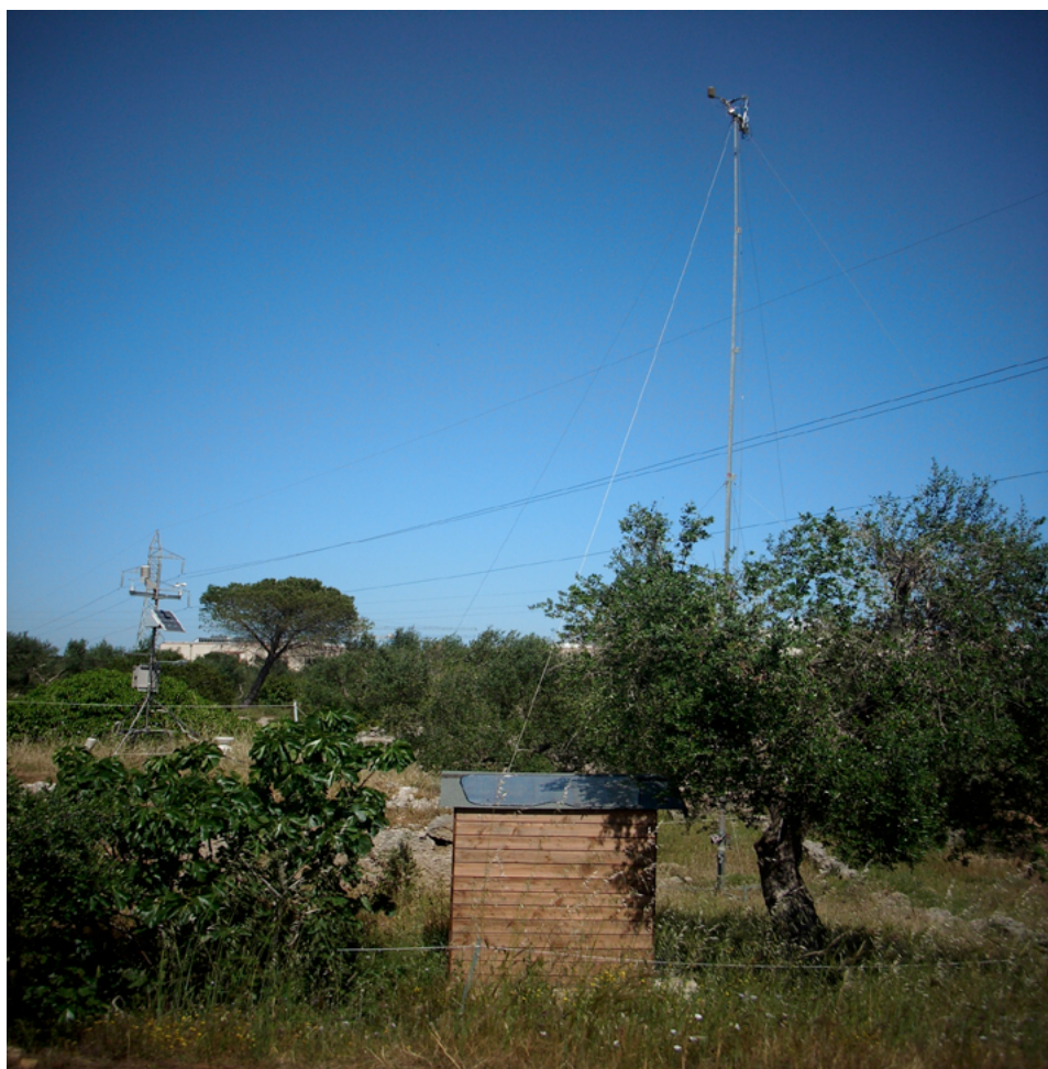
Fig. 2b: The ISAC base, from left: meteorological automatic station, computer shelter, micrometeorological mast
